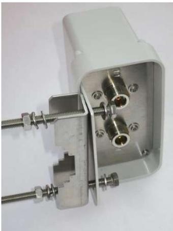
Step 2: Tighten inner nut
